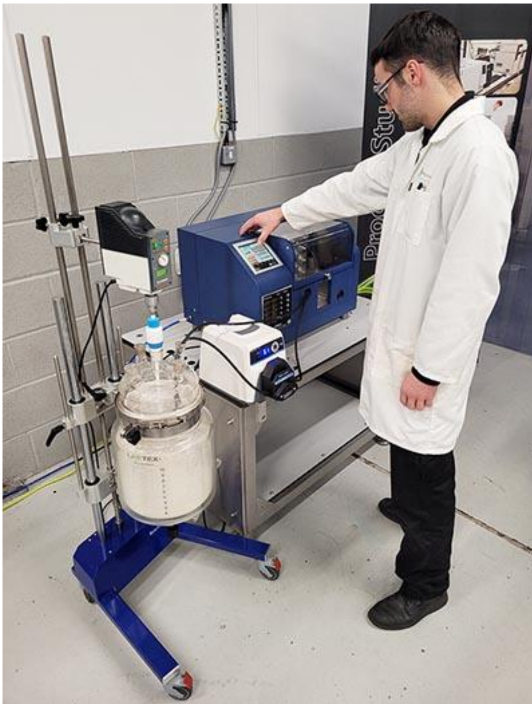
Image caption: AMT clean room operation using a Coflore® flow reactor fed by an efficiently stirred vessel in a ReactoMate ATOM stand.
