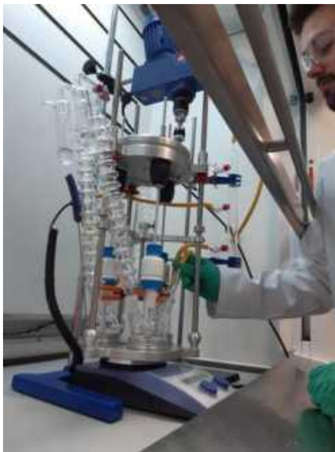
Images: DrySyn Vortex overhead stirrer with hotplate running 3 reactions in parallel
