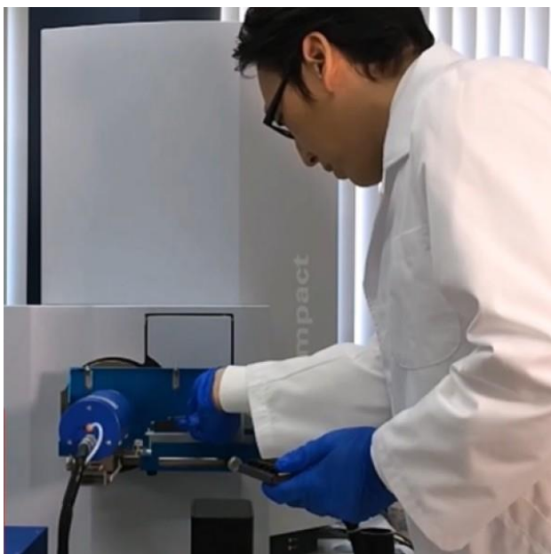
Caption: Introducing polymer sample into ionRocket temperature gradient sample introduction device for DART-MS
