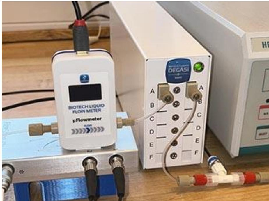
**Image caption:** Microflowmeter / Degasser set-up used in pharmaceutical formulation dispensing application
