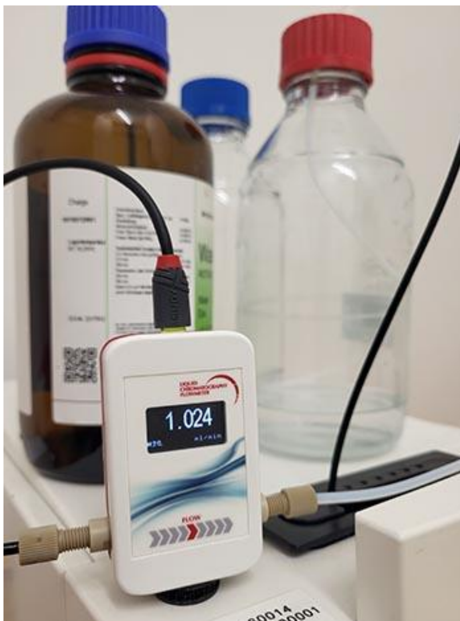
Image caption: HPLC system operation and performance qualification using a TESTA Analytical liquid chromatography
